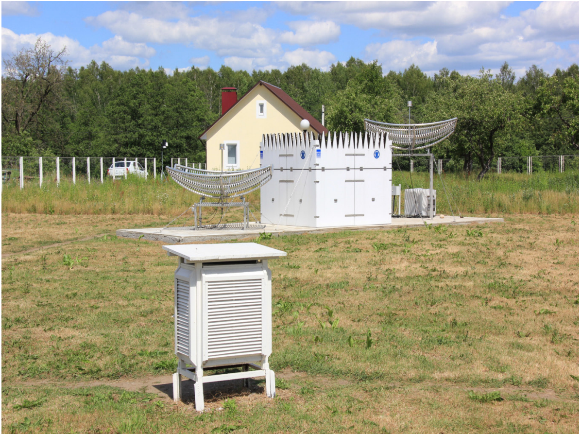
Figure 8.15 – SODAR measuring complex
