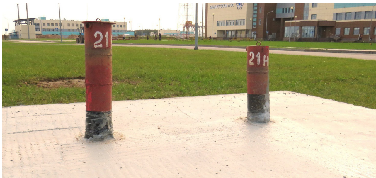
Figure 8.6 - Piezometric well cluster
